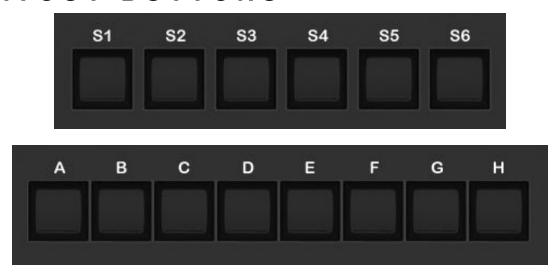
These 14 buttons are intended for frequently used functions in your software. If your controller does not support the **MIDICON-2™** as plug and play, you will have to link each button to a function using the setup menu in your software. Refer to your software instructions, as this will be different for each program. Please refer to the MIDI table at the end of this manual for each button's default MIDI note message.
