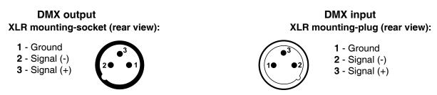
If you are using the standard DMX controllers, you can connect the DMX output of the controller directly with the DMX input of the first fixture in the DMX-chain. If you wish to connect DMX-controllers with other XLR-outputs, you need to use adapter-cables.
