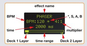
MIDI layers other than default Layer 1 are shown at the bottom of the effects display, Deck 1 on the
