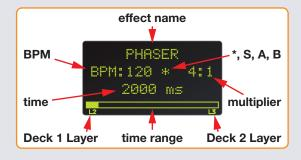
To change the BPM source, press and hold the **TAP** button and use the **BEAT** joystick to step through the sources. If a new BPM is manually tapped in or the time is manually altered, the BPM source returns to (\*) Manual.
