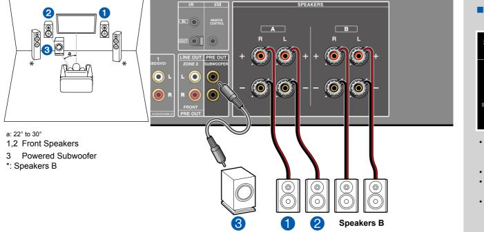
Along with the 2.1 Channel System (SPEAKERS A) ( $\rightarrow p21$ ), you can connect one more set of front speakers to use as a Speaker B System.
