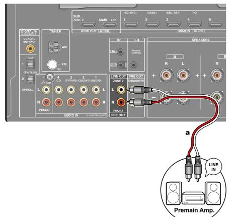
You can enjoy 2-ch audio in the separate room (ZONE 2) while performing playback in the main room (where this unit is located). Use an analog cable to connect the ZONE 2 LINE OUT jack of this unit and the LINE IN jack of the premain amplifier in the separate room. The same source can be played back in the main room and ZONE 2 simultaneously. Also, different sources can be played back in both rooms.
