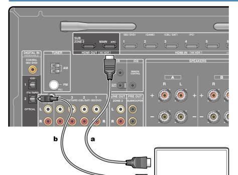
If the TV does not support the ARC (Audio Return Channel) function (\*), connect an HDMI cable and digital optical cable.
