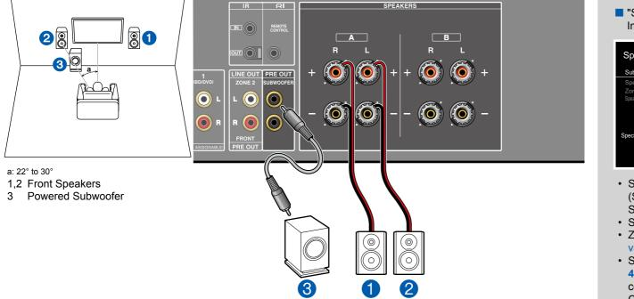
Front speakers output front stereo sound. The powered subwoofer reproduces bass sounds and enriches the sound field. The optimal positioning for front speakers is ear height. Placing the powered subwoofer between the front of the listening position and a front speaker gives you a natural sound even when playing music.
