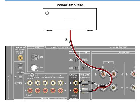
You can connect a power amplifier to the unit and use the unit as a pre-amplifier in order to produce a large volume that cannot be output with the unit only. Connect the front speakers to the power amplifier. For details, refer to the power amplifier's instruction manual.
