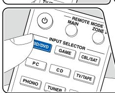
To return the remote controller to main room control mode: Press REMOTE MODE MAIN on the remote controller.
