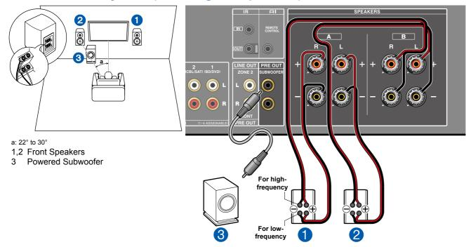
You can connect speakers that support bi-wiring to this unit. Connect the treble and bass correctly. Be sure to remove the jumper bar connecting between the woofer jacks and tweeter jacks of the Bi-wiring supported speakers. Refer to the instruction manual of your speakers as well.
