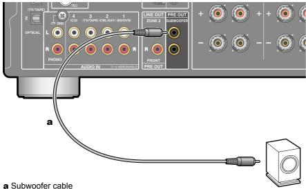
Connect a powered subwoofer with this unit using a subwoofer cable. Up to two powered subwoofers can be connected. The same signal is output from each SUBWOOFER PRE OUT jack.
