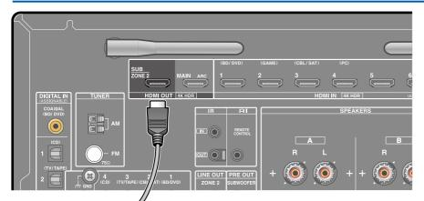
While a disc is played on a Blu-ray Disc player in the main room (where this unit is located), you can play the video and audio of the same Blu-ray Disc player or another AV component on the TV equipped with an HDMI IN jack in a separate room (ZONE 2). Note that only the devices connected to the HDMI IN1 to IN3 jacks can be played on the TV in the separate room.
