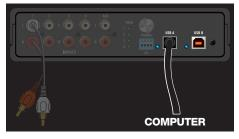
Using the provided USB cable, connect either USB A or USB B on your SL 4 to an available USB 2.0 port on your computer.
