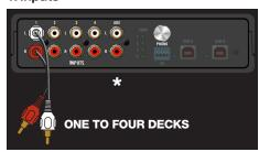
Connect your CD players or turntables to the SL4 INPUTS. If you use turntables, connect their ground wires to the ground terminal on either the SL4 or your mixer. \*Optional Step: Connect an additional output (such as AUX OUT) from your mixer to the AUX INPUTS on the SL4 to record your set in Scratch Live. See "Recording" on page 29.
