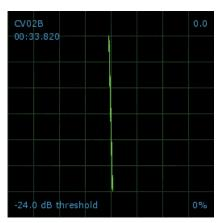
**LEFT CHANNEL MISSING** - The signal from the needle is not reaching the SL4. Check the cable and cartridge connections.
