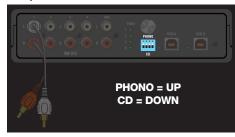
Set each input to the correct input level using the dip switches. Set the switches UP for Phono (turntables) or DOWN for CD players (line level).
