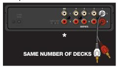
Connect the OUTPUTS of the SL4 to Linelevel inputs on your mixer. \*Connect the AUX output to an additional line or AUX input on your mixer to output the sample player. See "SP-6 Sample Player" on page 20.
