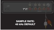
Use this to switch between 48 kHz and 96 kHz. Use 48 kHz by default if you are not using 96kHz audio files.
