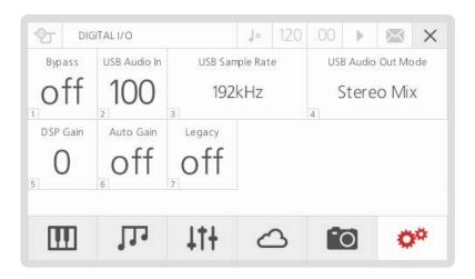
USB audio-out is available using 4 different sample rates, which each appear on the host computer as separate USB devices/drivers. These are:
