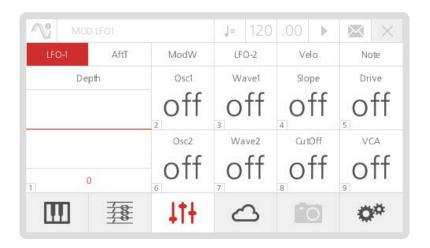
Individual modulation depths provided for all LFO2 destinations: to change the modulation amount for a specific destination, please hold down the destination button and turn the 'Depth' knob on the front panel.
