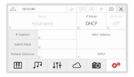
The IP Mode area displays 'DHCP' and your 002 should have an automatically assigned IP Address: a valid local IP address has the 192.168.0.x format.
