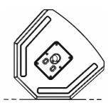
The rear side inclination, symmetrical, as shown in the upper picture, is 45°. SYA15 can be used as a stage monitor in small contexts, in this case please consider the characteristic dispersion pattern presented above.
