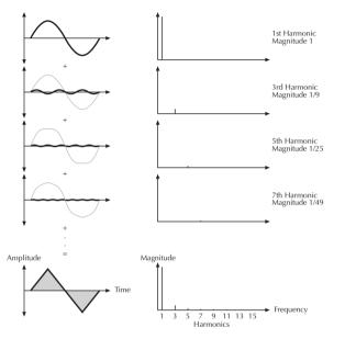
Additive components of the Triangle wave
