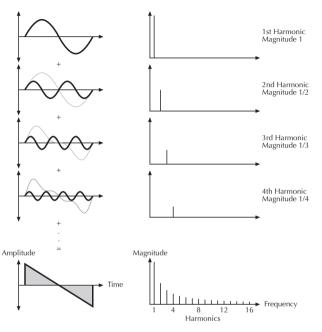
Additive components of the Sawtooth wave
