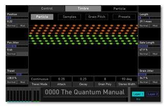
The Particle parameter page can only be reached, if the Mode is set to 'Granular'. This can be done by tapping on the **Particles** button (and confirming the granular mode switch) or selecting *Granular* with the **Mode** parameter.
