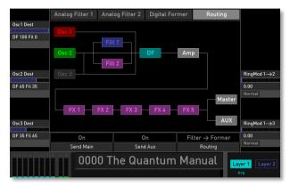
Here you will get a graphic overview of the Quantum's signal routing. You can also control the routing of the three oscillators, the ring modulators, and set up the audio outputs for the current sound.
