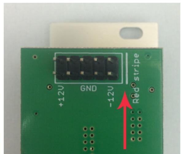
Most modules will come with the cable already connected but it is good to double check the orientation. Be aware that some modules may have headers that serve other purposes so ensure the cable is connected to the right one.
