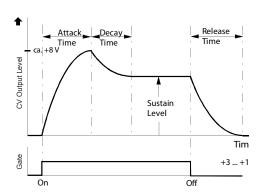
As soon as the envelope generator receives a gate-on signal, its output CV will rise from 0 Volt to maximum. The rise time is adjustable and called "Attack". When the maximum value has been reached, the voltage will drop within a timespan defined by the "Decay" pot to the "Sustain" level. The envelope control voltage will stay on this level until the key is released, then it will drop to 0 Volt within the "Release" time dialled up.
