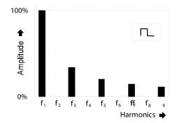
The width of a pulse wave can be modulated by a low frequency oscillator (LFO) or, less common, by an envelope generator. This way the harmonic spectrum of the pulse wave does not remeain static. The resulting sound is similar to the chorusing effect between two oscillators which are nearly perfectly in tune, i. e. unison. The modulation frequency has to be very low (approx. 1 Hz or lower) because otherwise the oscillator will sound out of tune.
