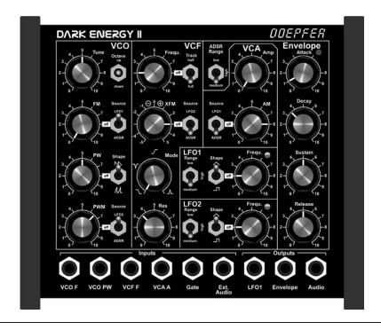
As soon as the power adaptor has been plugged in, Dark Energy II will power up. The LEDs in both LFO sections will now light up and alternate between red and green. The LED on the back panel will flash intermittently for about two seconds and then stay lit permanently.
