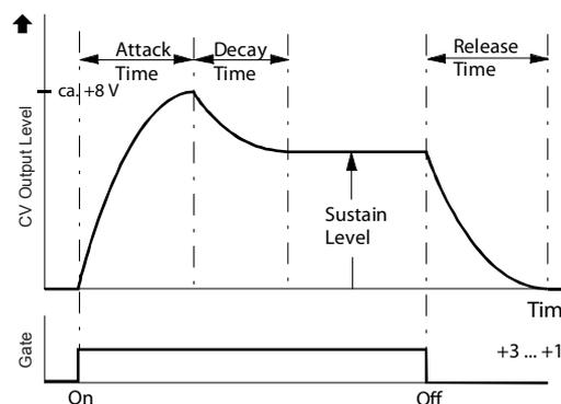
As soon as the envelope generator receives a gate-on signal, its output CV will rise from 0 Volt to maximum. The rise time is adjustable and called „Attack“. When the maximum value has been reached, the voltage will drop within a timespan defined by the „Decay“ pot to the „Sustain“ level. The envelope control voltage will stay on this level until the key is released, then it will drop to 0 Volt within the „Release“ time dialled up.
