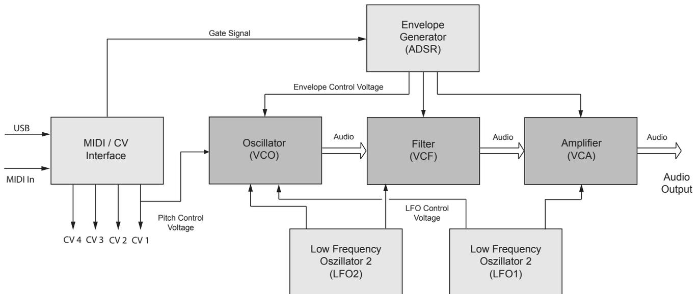
The figure above illustrates an overview of Dark Energy III's signal path.
