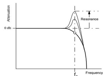
The resonance characteristics of a lowpass filter
