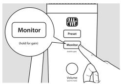
Press the Monitor button and turn the knob to adjust the blend
