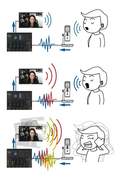
Whenever you're recording using the Revelator mixer with an application that offers monitoring, like Studio One or OBS, you must either disable monitoring or mute the return channel in your Revelator mixer to avoid creating a feedback loop.
