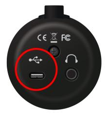
**USB-C Compatible Connection.** Use this port to connect your Revelator to your computer. While the Revelator's onboard connection is USB Type C, it is fully compatible with USB Type A 2.0 and 3.0 connections. Use the USB-C to A cable that came with your Revelator if your computer has a USB-A connection rather than a USB-C connection. Please note: *Revelator is backward compatible with USB 2.0 and USB 3.0 speed connections. USB 1.1 is not supported.*
