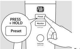
To bypass the presets, just press and hold the Preset button. The button will illuminate red while presets are bypassed.
