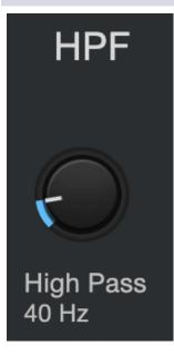
Use this control to set the High-Pass Filter frequency threshold for the selected Channel or Output Bus. The filter's threshold can be set from 24 Hz to 1 kHz. When the threshold is set to its lowest point, the filter is off. The highpass filter's slope is -12 dB/8va.
