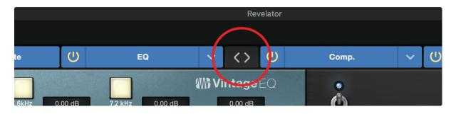
*Power User Tip:* Placing the compressor before the EQ allows you to make dramatic changes to the EQ settings without needing to alter the compressor setting. However, if you place the EQ before the compressor, you can better control different frequencies, achieving a more natural response.
