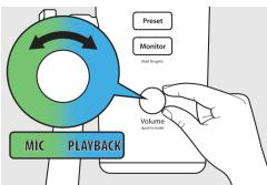
Turning the knob to the left will increase the level of the input
