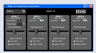
**Phono Sensitivity**: If Phono Input is selected on the mixer (as shown for Deck 3) the Phono Sensitivity adjustment appears in the panel. Click the down-arrow to display a list of 16 sensitivity settings between 2.5 mV and 10 mV in 0.5 mV steps. The default is 5 mV. Set the Phono Sensitivity to the same level of your cartridge (see your cartridge documentation for the correct value). Another method is to match the level of a CD on another input.
