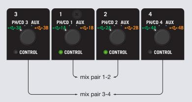
The source selectors choose the active USB port, USB audio slot or analog input for each input channel.
