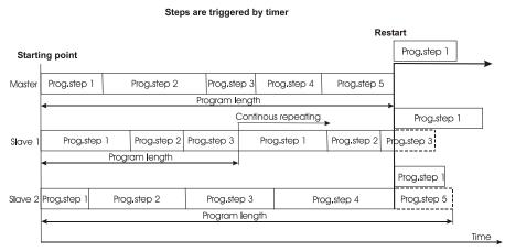
finishes its own program and restarts its program running (slave 1- prog.step 3 will not be finished). If the slave fixture has a longer program length, it will restart at prog. step 1 before it completes all its prog.steps
