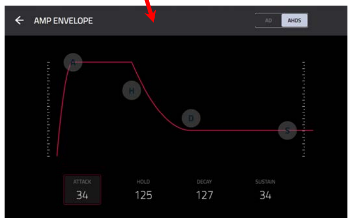
Close-up of an AHDS-type amp envelope.
