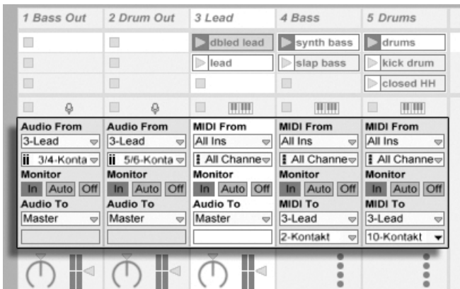
Tracks Feeding MIDI to and Tapping Audio From the Parts of a Multi-Timbral Instrument.
