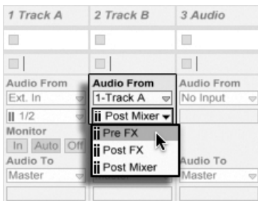
Tap Points for Track Routing.
