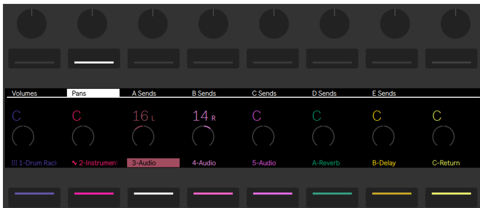
Controlling the Pans for Eight Tracks.
