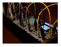
Connect a MIDI controller to the MIDI In jack to trigger pads and modulate parameters. Use the included Mini-TRS to MIDI 5-PIN DIN adapter if needed. This TRS jack supports both Mini-TRS type A and Mini-TRS Type B connections.
