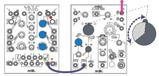
Figure 20: Subtracting the MATHS unipolar voltage to the Echophon's Pitch Panel Control Offset, using the Pitch1 Input Attenuvertor to invert the signal's polarity. The resulting "range" of movement is indicated by the crosshatched are of the Pitch Panel Control.
