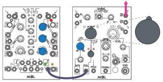
Figure 19: With the Pitch1 Input Attenverter set to 12 o'clock, no voltage is added to the Echophon's Pitch Panel Control setting and therefore does not move.
