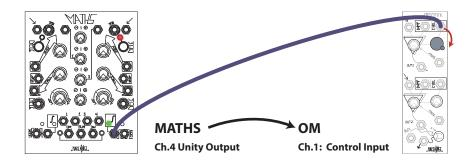
Have a look at the CYCLE button for MATHS Ch. 4. It has a Red LED next to it to indicate whether the Channel is **Cycling**.<sup>3</sup> If it's not, [PRESS] the Cycle button.
