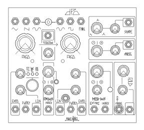
The DPO, as previously mentioned, is the primary sound source of the Shared System. It contains two voltage-controlled oscillators (VCOs) that are both independent and related. The two oscillators each have their own section on the faceplate, VCO A on the left and VCO B on the right. The two oscillators have identical cores, but some differences in function.
