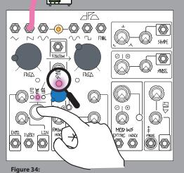
VCO A: Sawtooth Wave Output (Before Sync Is Engaged)
