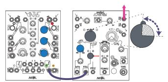
Figure 18: Adding the MATHS unipolar voltage to the Echophon's Pitch Panel Control Offset. The resulting "range" of movement is indicated by the crosshatched are of the Pitch Panel Control.
