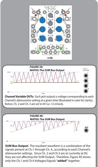
Notice: the output clips as soon as the Voltages reaches +10V, as the SUM Bus Output can not be greater than +10V or less than -10V.
