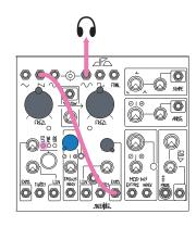
Engage LFO on VCO A VCO A SAW -> VCO B Expo FM In VCO B Sine -> Monitor Adjust FM Bus Index panel control Full CCW. Adjust both frequency knobs to ~12:00. Adjust VCO B Expo FM Input attenuator gradually clockwise.
