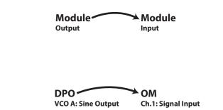
This is instructing you to patch the Sine Wave Output of the DPO's A oscillator to the signal input on Channel 1 of the Optomix. Don't worry if it sounds daunting, you'll quickly get the hang of it. Accompanying the written patch instructions, you'll also find small, visual representations of the connections. Continuing the example above:
