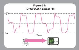
**The Exponential FM** Input has a different response: the Modulation Depth is more drastic the higher the input voltage. Thus, the response is greater to positive CV than it is to negative CV: the negative portion of the modulating waveform does not slow the VCO down by nearly as much as the positive half speeds it up.
