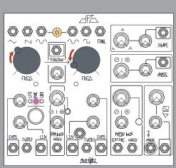
VCO A also has a behavior called **Follow**, accessed via the Follow Panel Control and CV input between the two grey frequency knobs. When Follow is turned up all the way, VCO A will "follow" any Control Voltage signal present in VCO B's 1V/Octave CV input.
