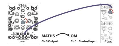
Channels 2 and 3 of MATHS generate voltage **Offsets**. An Offset is a constant voltage at a level set by the panel control. As you turn up the panel control for MATHS Ch.3, its Offset goes from 0v up to +5v, and you should hear a resulting increase in the amplitude of the sound going through the Optomix. (Note: this Offset is only generated if there is NO patch cable in the MATHS Ch.3 Input.)
