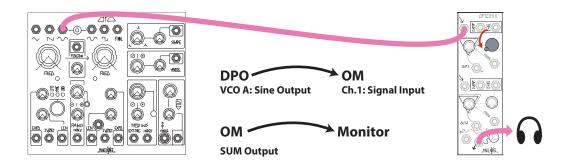
In case you missed the explanation above or need a refresher, this diagram is instructing you to patch the SINE Output of VCO A (it's a curvy wave, as opposed to the pointy triangle and sawtooth) into the Signal Input of Channel 1 of the Optomix (the top left jack). Now, Adjust the Optomix's Ch.1 Panel Control (top right knob) to full CCW.
