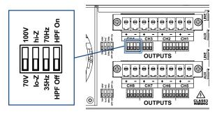
FIGURE 17: Rear output connection and DIP switch.
