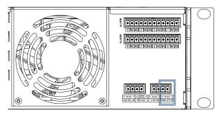
FIGURE 20: Remote on/off switch connector.
