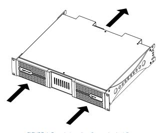
FIGURE 6: Forced air cooling: front to back airflow.
