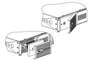
FIGURE 8: Magnetic side panel removal.
