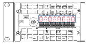
FIGURE 9: Front panel pot attenuators.
