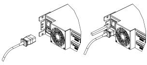
FIGURE 7: Mains connector and on/off power switch.
