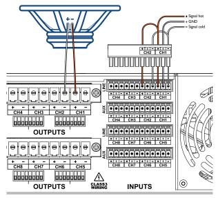
FIGURE 18: Output BRIDGE connection; Input PARALLEL connection.
