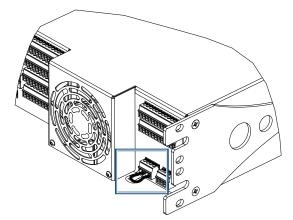
FIGURE 14: AUX SEL and PWS OUT jumper.
