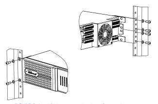
FIGURE 5: Amplifier's mounting brackets; front and rear view.
