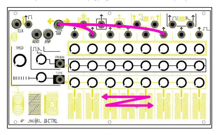
There are eleven touchplates on the 0-CTRL: three for macro control, and eight for Step selection and generating Pressure and Touch Gate signals.
