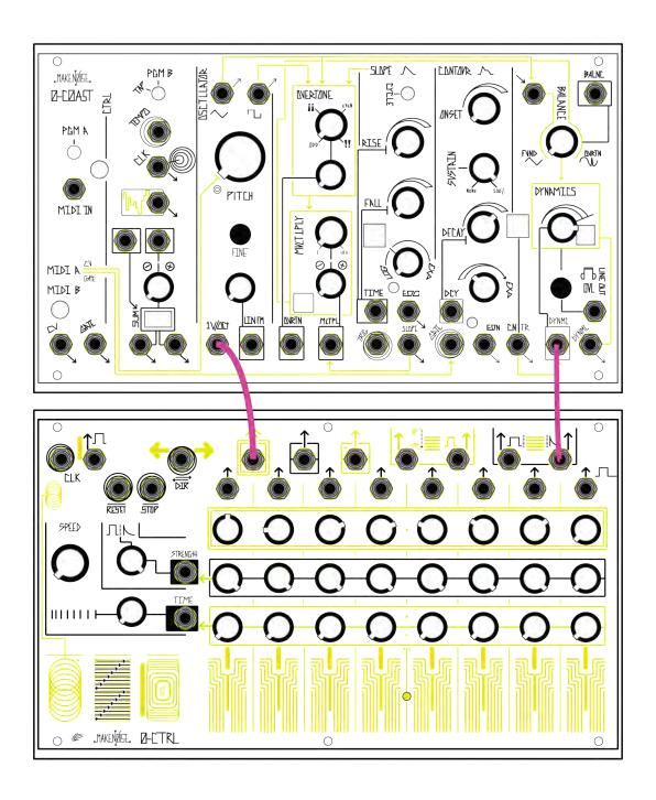
Once you have made these initial connections and settings, start the Clock using the Clock touchplate (the CLOCK Window will light white to show that the Clock is going, and the Step Indicator lights will start to "move" as they are sequenced).
