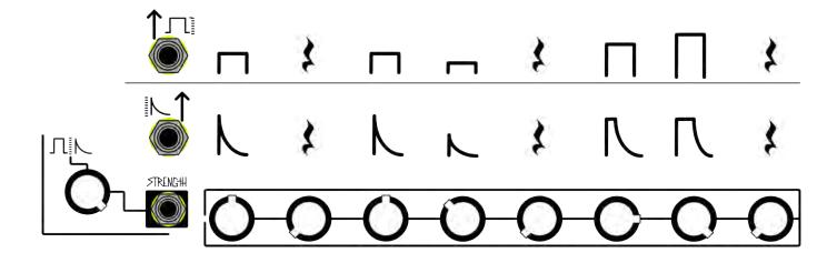
When the Time attenuator is turned up, the Time row will set the Clock Rate per step, and thereby the length of each note in the sequence. The resulting setting is not quantized in any way, allowing for any rhythm to be created, on or off "the grid." (Diagram for illustration purposes, not to scale)
