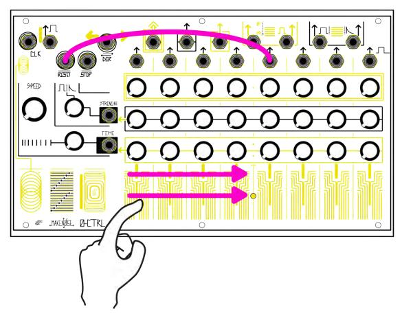
A gate to the Stop input will cause the sequence to stop until the gate goes low again.\* Patch a Step Gate Output to this input to create "one-shot" sequences. Touch a Step touchplate to "fire" a sequence, which will stop when it reaches the Step whose gate was patched to Stop.
