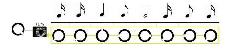
In addition to their control of Dynamics and Rhythm for the 0-Ctrl's sequencer, the Strength and Time Channels each have a sequence CV output, located next to the Pitch channel's CV output, which can be patched to any voltage-controllable parameter for sequencing of timbre, pitch of a second or third VCO, etc.
