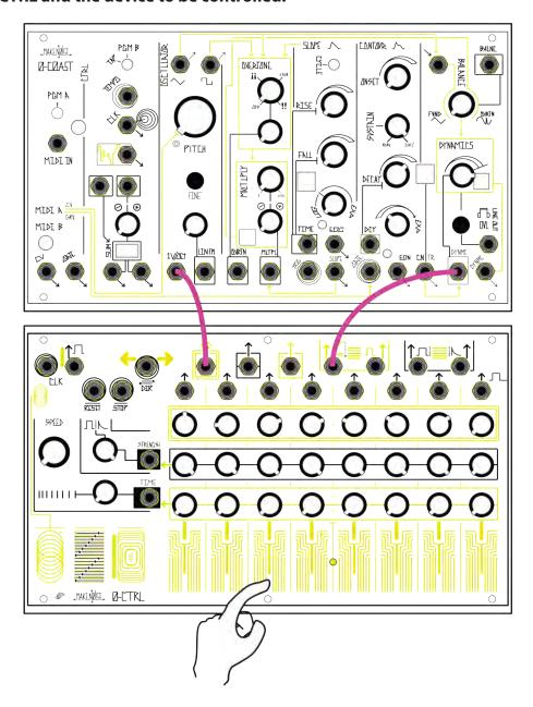
Alternatively, you can patch the Touch Gate to the Contour Gate Input for envelope generation instead of direct pressure voltage.
