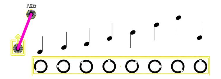
As with all the Channel outputs, the Pitch CV output can be patched to any voltage-controlled parameter, including but not limited to Pitch. Use a stacking patch cable to send it to multiple places.
