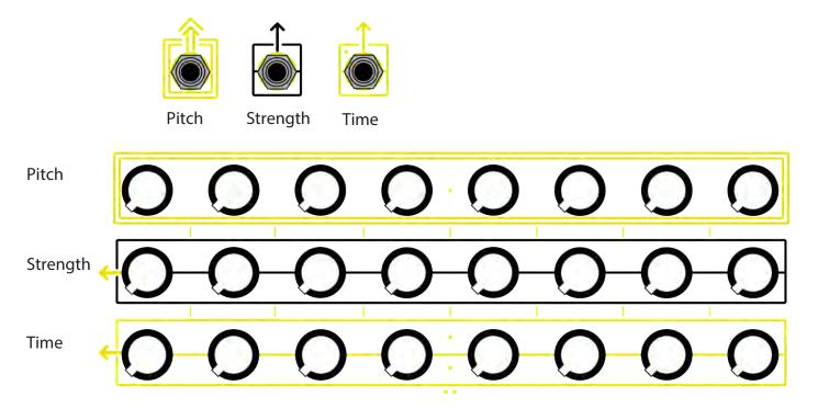
Like many classic sequencers, the 0-CTRL is a 100% analog device, and therefore has no pitch quantization on its CV outputs. They can certainly be used to control the pitch of oscillators, but there is no arbitrary limit to the precision of values they can create. Instead, the 0-CTRL encourages you to use your hands and ears to find frequencies, and your imagination to decide where to patch this control voltage.
