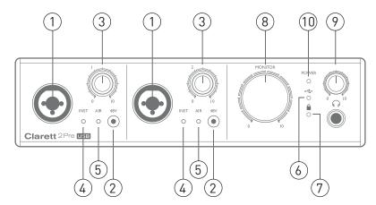
The front panel includes the input gain controls and input connectors for Mic, Line and Instrument signals for both channels, and also the monitoring controls.
