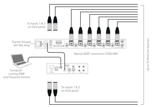
The Clarett OctoPre's **OPTICAL OUT** port is connected to the Clarett 2Pre USB's **OPTICAL IN** port with a single TOSLINK optical cable. The two devices must be synchronised to ensure audio passes cleanly, without clicks and pops. This can be achieved by selecting ADAT as the clock source in the **Device Settings** tab within the Focusrite Control software. Both devices must be set to the same sample rate."
