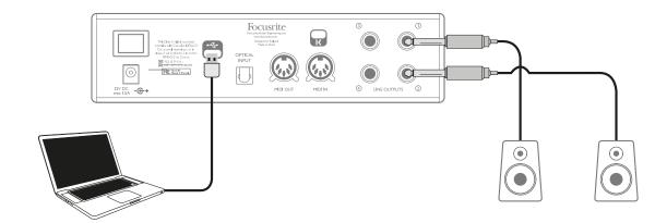
This setup illustrates a typical configuration for multitrack recording with DAW software on your computer.
