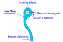
CAUTION: DO NOT attempt to rotate the Clamp Lever exceed from the maximum clamping point. It will loosen the clamping pressure.
