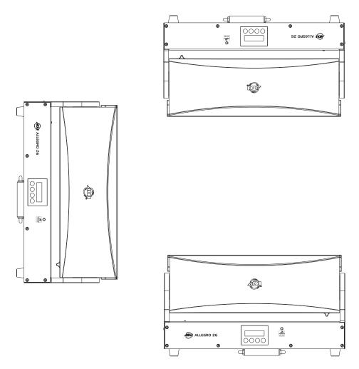
The Allegro Z6 is fully operational in three different mounting positions, hanging upside-down from a ceiling or trussing, sideways on trussing, or set on a flat level surface. Be sure this fixture is kept at least 12m (40ft) away from any flammable materials (decoration etc.). Always use and install the supplied safety cable as a safety measure to prevent accidental damage and/or injury in the event the clamp fails (see next page). Never use the carrying handles for secondary attachment.
