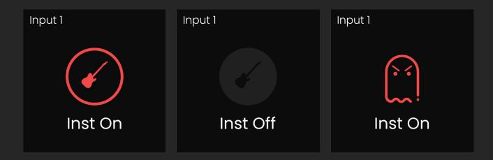
If you try and activate phantom power on Channels 1+2 whilst the instrument input is active, an error screen will be shown as it is not possible to have both active at once.
