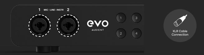
To connect a microphone, use an XLR cable which has three pins.
