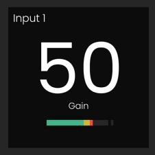
When pressing an Input Button, the status screen will display: the input number, the gain setting in dB, and an independent channel meter for referencing your levels.
