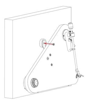
We recommend using the appropriate type of mounting screw for given type of the wall.
