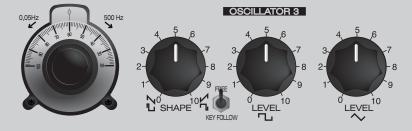
the patch matrix, the triangle output shares the input with the Sample&Hold output. Use the switch on the Sample&Hold module to select the output, which is routed to the matrix! Set the master frequency for Oscillator 3 Adjust the waveshape for both waves simultaneously Use the switch to choose between a free running or CV controlled mode
