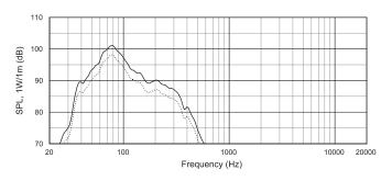
SB-2 frequency response, (1W total, 1m) at two-boundary junction ( $\pi$  loading, dotted line) and at three-boundary junction ( $\pi$ /<sub>2</sub> loading, solid line).
