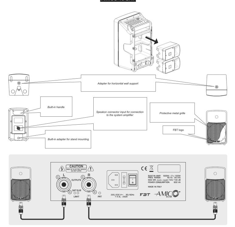
The satellites are designed to be installed on floor stand; such installation will allow medium-high frequency sources to be better aligned to listener's ear.
