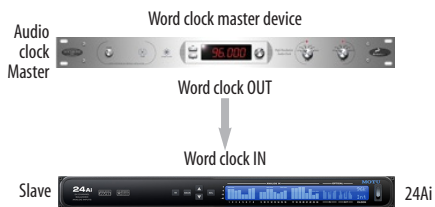
Figure 4-9: Slaving your MOTU device (a 24Ai in this example) to word clock. For the 24Ai clock source, choose 'Word Clock In'.
