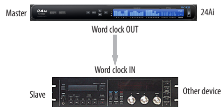
Figure 4-8: Slaving another digital audio device to your MOTU device (a 24Ai in this example) via word clock. For the 24Ai clock source, choose any source besides word clock, as it is not advisable to chain word clock.
