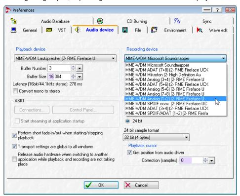
Increasing the number and/or size of audio buffers may prevent the audio signal from breaking up, but also increases latency i.e. output is delayed. For synchronized playback of audio and MIDI (or similar), be sure to activate the checkbox 'Get position from audio driver'.
