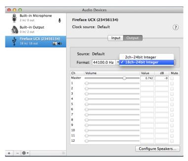
Mac OSX supports USB Audio 2.0, even with more than 2 channels. The UCX offers 18 input and 18 output channels at up to 96 kHz. It is shown as "Fireface UCX (xxxxxxxxx)" in the Audio MIDI Setup, in both normal and CC mode. In CC mode the USB Settings will vanish from the Dock, and TotalMix will – if at all – show a 'disconnected' UCX.
