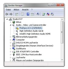
Windows does not support USB Audio 2.0 directly. The UCX will be detected, but automatic driver installation will fail. This is important to remember. Connecting it to the PC one day after having it used with the iPhone/iPad one might forget that it is still in CC mode. You might end up with hours of wasted time trying to repair your driver installation – when all you need to do is set the unit back to normal mode.
