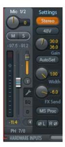
Width. Defines the stereo width. 1.00 equals full stereo, 0.00 mono, -1.00 swapped channels.
