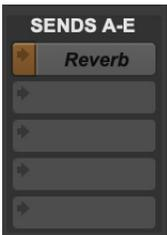
*DSP Mode-enabled, send inactive due to insufficient resources*
