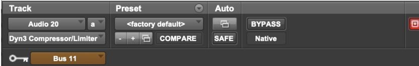
*DSP Mode, Key Input inactive due to insufficient DSP resources*
