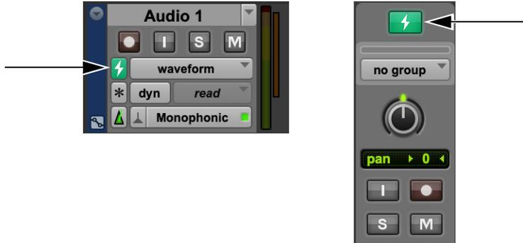
Track DSP Mode button enabled: in the Edit window (left) and in the Mix window (right)
