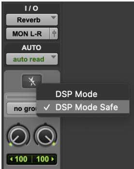
Enabling DSP Mode Safe on a track in the Mix window
