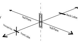
The sound of your R84 series microphone is slightly different between the front and the back – subtle, but sufficient to offer two "flavors." In addition to polarity, this is the result of using two wraps of grille cloth on the back and only one on the front. When using the rear lobe, remember to invert the polarity on your preamp or DAW. This ensures your recordings with the back lobe will be inphase with other microphones.
