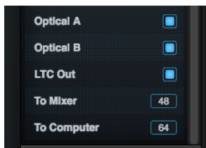
Figure 10-2: The 'To computer' setting (item 30 on page 15) determines how many channels you see in the Left Input and Right Input menus.
