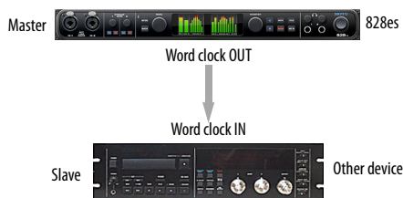
Figure 5-20: Slaving another digital audio device to your MOTU device (an 828es in this example) via word clock. For the 828es clock source, choose Internal . Alternately, the MOTU interface could be resolved to any other external clock source besides Optical , except for Word Clock , as it is not advisable to chain word clock.
