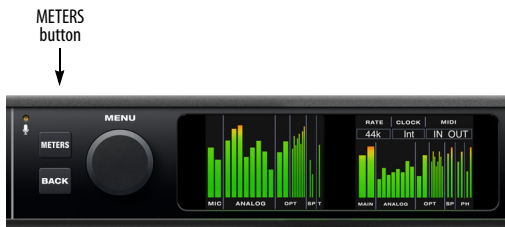
Figure 7-1: Push the METERS button to cycle among three LCD screen sets that provide extensive metering, activity indicators and status information.
