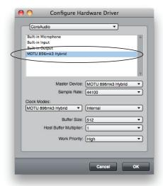
Figure 7-2: Enabling the 896mk3 Hybrid in Digital Performer
