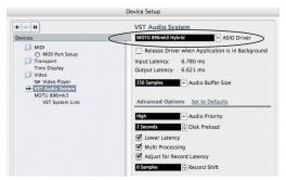
Figure 7-7: Enabling the 896mk3 Hybrid in Cubase
