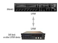
896mk3 Clock Source setting = Internal (when transferring from the 896mk3 to the S/PDIF device) 896mk3
