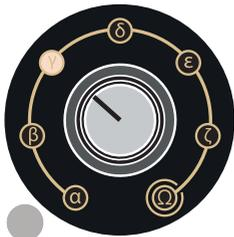
Move layer knob to desired location to select record and playback layer (illuminated off white).
