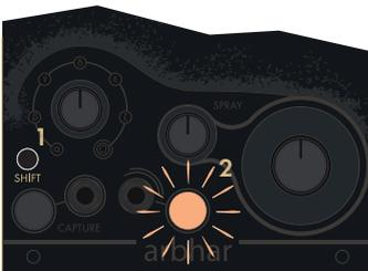
To undo an overdub hold 1, press 2. When pulsing orange the action will undo.
