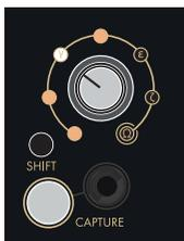
**Gamma:** The gamma setting will not activate capture upon onset detection.
