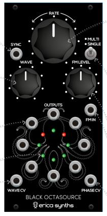
Use large knob to control LFO rate manually! 12 o'clock position will "freeze" all momentary CVs on the outputs. Turning the knob clockwise will gradually increase LFO frequency, and the phase shift will occur in CW direction. Turning the knob counter clockwise will gradually increase LFO frequency, and the phase shift will occur in CCW direction.
