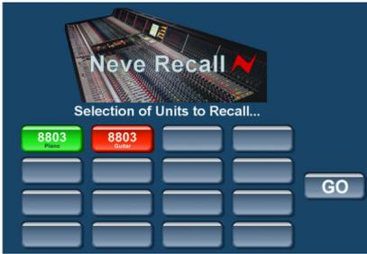
Neve Recall software allows settings from the 2254/R to be stored on a PC or Mac and recalled for later use.
