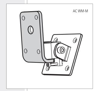
It is possible to fix the moving part of the AC WM-M accessory directly to the loudspeaker rear panel (in one of the possible positions), through four M6 flat head screws (as shown in the figure below).
