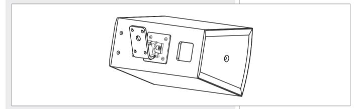
Then, put the loudspeaker on the fixed part of the AC WM-M accessory (that is wall-mounted) and tighten the bolt. The screw below allows vertical tilt adjustments.
