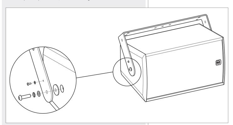
Before tightening the two M10 bolts, adjust the loudspeaker vertical tilt and then fix it through two M4.2x22 self-threading screws (passing through the small hole of the U bracket) directly into the loudspeaker cabinet wood.
