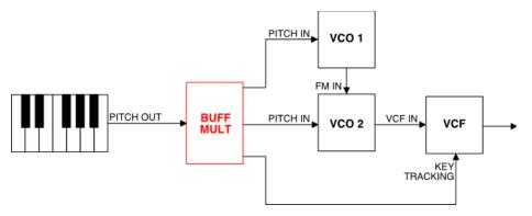
Unlike a passive mult, which merely splits the incoming signal and shares it across multiple outputs (much like a Y-cable), buffered mults make electrical copies of an input voltage and duplicate that voltage at the outputs.
