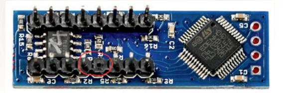
Install the new Core in the socket and press on it with thumbs of both hands tightly to ensure it is installed fully. There still should be like 3mm pitch between the socket and plastic housing of the Core pins.
