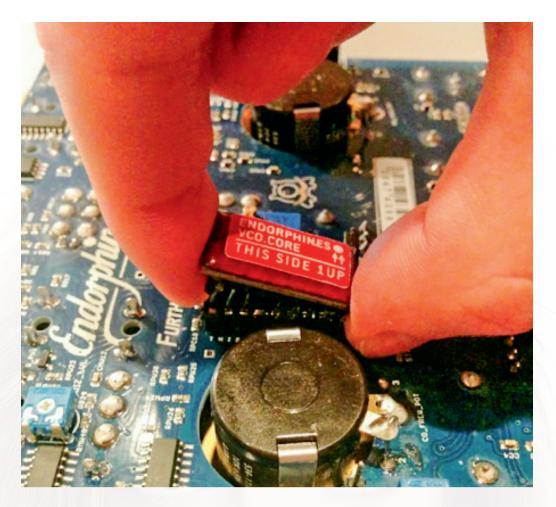
Each VCO Core has white round pin at one of its edges that defines the first pin and its orientation. Moreover, there is one pin of the Core missing and one pin in the socket is covered with soldering acting together as a key, so it is literally impossible to plug the Core in the wrong way backwards.
