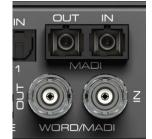
Selecting *Single Speed* in the Settings dialog causes the output signal to always stay within the range of 32 kHz to 48 kHz. So at 96 kHz and 192 kHz sample rate, the output word clock is 48 kHz.
