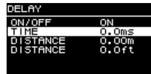
To edit parameters that have continuous values, turn the main knob to change the value for that parameter. The value is changed in real time as you turn the knob.
