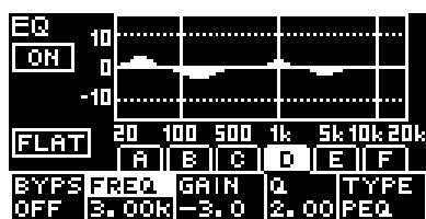
Configure the equalizer settings. The total gain characteristics for a 6-band equalizer are displayed on a graph.
