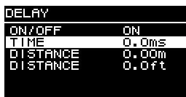
Allows you to switch the delay ON or OFF, and configure three types of delay settings. Editing one type will affect the settings for the other types.
