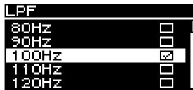
Configure the low-pass filter frequency settings.
