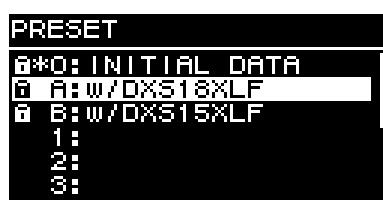
Allows you to store up to eight sound-related settings. When using the DZR and DXS-XLF series, simply recalling the preset of the speaker model to be used optimizes the corresponding settings. Recalling INITIAL DATA allows you to return to the factory settings.
