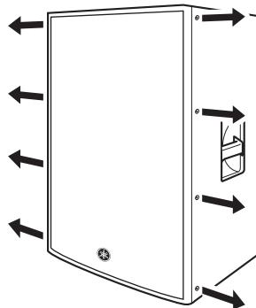
2. Using a No. 2 Phillips head screwdriver, remove all screws installed on the horn and pull the horn out from the speaker.
