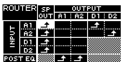
Configure the routing of the audio signal. Set for the routing point of the signal you want to output. You can set the input and output levels by selecting INPUT or OUTPUT and going to the INPUT or OUTPUT level setting screen.
