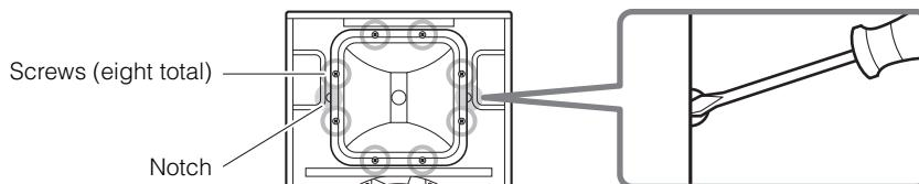
3. Rotate the horn 90 degrees, and re-install the horn to the speaker, reversing the steps above.
