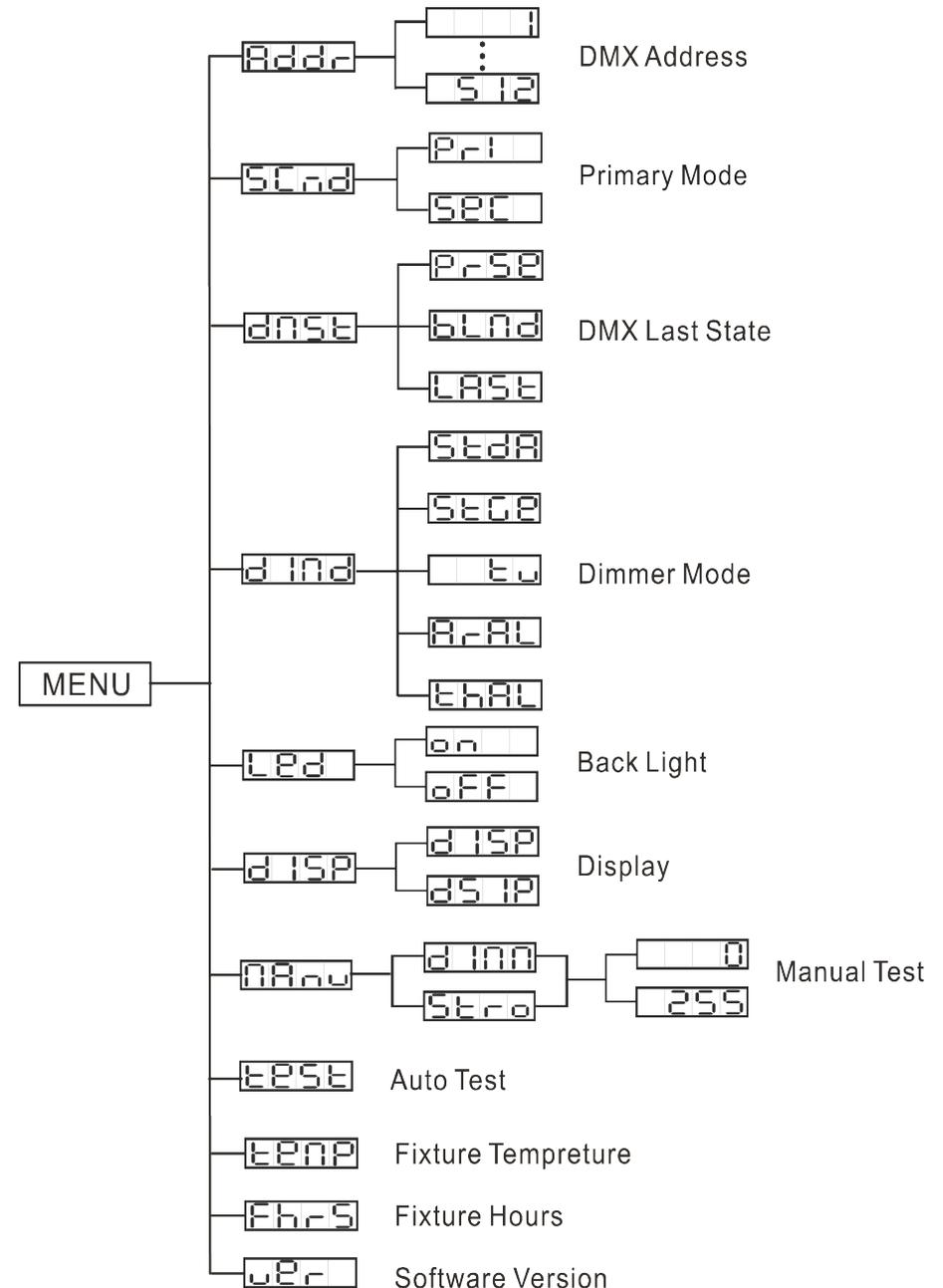
**On-Board System Menu.** The Ikon Profile comes with an easy to navigate system menu. This next section will detail the functions of each command in the system menu. **Please read the next section thoroughly!**
