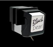
Type: MM Frequency Response: 18Hz - 27kHz Output Voltage: 4.0 mV Load Impedance: 47k ohms Channel Seperation: 28dB at 1kHz Channel Balance: 0.5 at 1kHz Stylus Type: Spherical Compliance: 15 x 10<sup>-6</sup> cm/dyne Tracking Force Range: 1.5 - 2.0 grams Recommended Force: 2.0 grams
